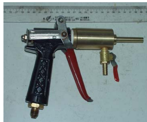
Fig. 3. Outline of the new squirt gun for cleaning.
